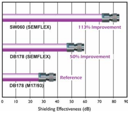
SEMFLX vs RG178: SHIELDING EFFECTIVENESS (% improvement with respect to RG178)
